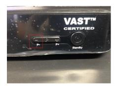
Hold down the P- button on the front of the satellite box and then plug the power lead back in whilst continuing to hold the P-button. When you see the firmware download screen appear on your tv screen you can let go of the P- button.
