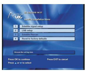
Press OK on "Satellite Rescan" to rescan the decoder with the new LNB settings.
