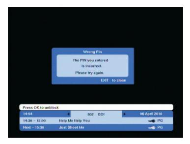
After the third incorrect pin entry, the pin code is locked, you must then do a factory reset of the STB in the Menus.
