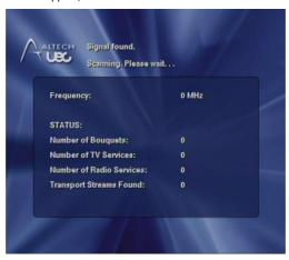
If 'Signal Found' is displayed at the top of the screen then the unit will begin to scan in services and channel 800 will appear.
