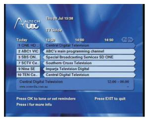
Use the arrow buttons on the remote to scroll through the TV Guide grid. The "P+/P-" buttons will move the grid right/left by 24 hours.
